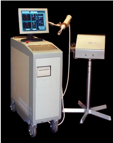
Figure 1: The Sonablate™-500 HIFU device with a transrectal probe attached to an articulated arm. The arm is fixed to an operating table and the user adjusts the probe position to optimize both imaging and treatment of the prostate. The active cooling device circulates cold water to keep the rectal temperature at a safe level. The device has both imaging and HIFU capability on the same transducer that ensures absolute coordination of imaging and treatment position to image and monitor tissue changes on each ablative pulse.
