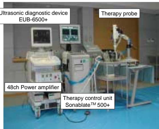
FIGURE 5. Construction of the therapy system FIGURE 6. Outline view of the therapy system
